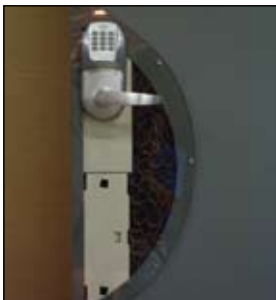
Hidden electronics provide added security and enhanced aesthetics (cutway shown).
