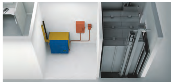
Conventional System: requires dedicated space for the elevator machine room.
