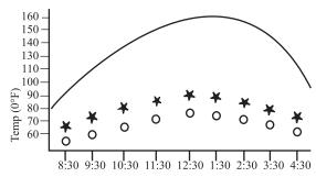
Black uncoated shingles White ROOF MATE coated shingles
