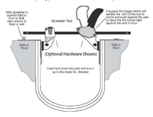
Step 5: Drill appropriate size holes at a maximum distance of 12"apart. Anchor the barrier to the concrete.
