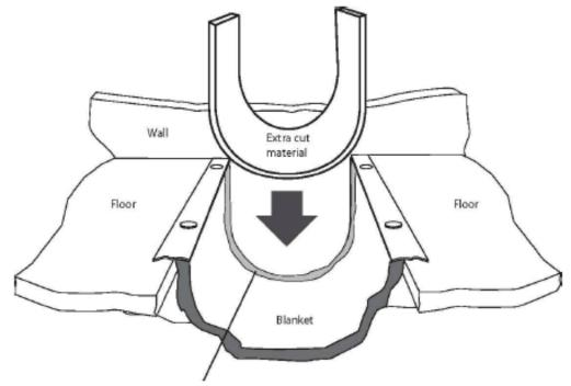
Caulk the cut M end to the wall. Make sure there are no holes or leaks.
