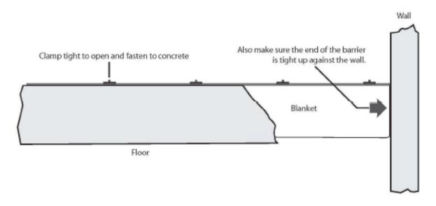
Step 3: Caulk the cut M end to the wall. Make sure there are no holes or leaks. It is estimated that the complete (entire) tube of calk is required for one end of a joint. Place the excess cut material over the caulked section.
