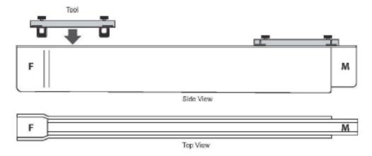
Step 3: Place the fire barrier in the expansion joint, Fireline 520\* blankets have a 12" overlap on each end. One end is a male (M), while the other end is a female (F). Start at the Female end of any directional changes as they should already be installed. Put a bead of caulk approximately 1" in from the end as stated in the general notes.
