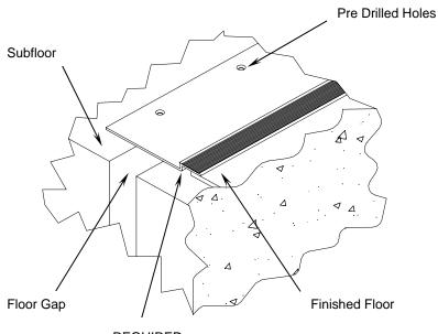
REQUIRED: INSTALL WITH OPEN SPACE TO ALLOW FOR FLOOR MOVEMENT
