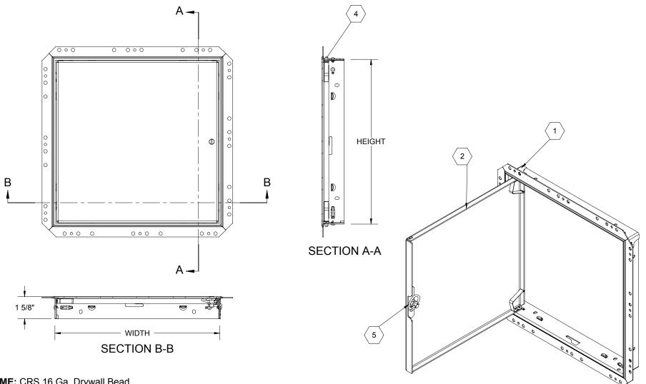
FRAME: CRS 16 Ga, Drywall Bead
