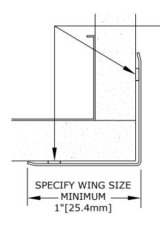
USE 1/4" [6.4mm] CONTINUOUS BEAD OF MASTIC ADHESIVE EACH FLANGE. SEAT FIRMLY ON FLOOR TO AVOID SLIPPAGE DURING SET-UP.
