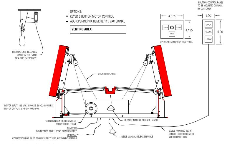
STANDARD CURB CONSTRUCTION IS INTENDED FOR INSTALLATION ON FLAT ROOFS ONLY. FOR A SLOPED ROOF APPLICATION PITCH CORRECTED OPTION MUST BE SELECTED.
