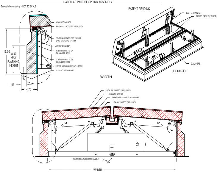
THE SMOKE VENT USES 110V AC TO ALLOW FOR MOTORIZED OPENING AND CLOSING OF DOOR LEAFS USING A 3 BUTTON CONTROL PANEL. THERMAL LINKS ON EACH LEAF ALLOW AUTOMATIC OPENING IN CASE OF A FIRE EMERGENCY. INCLUDES TERMINALS FOR REMOTE 24VDC SIGNAL TO OPEN DOORS. MINIMAL & OBSTRUCTED CLEAR OPENING.
