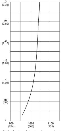
Free Area Velocity in feet and (meters) per minute Standard air .075 lb/ft<sup>3</sup>
