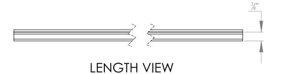
OUR QUIETFLEX ENTRANCE MATS HAVE RECYCLED LOW-DENSITY POLYETHYLENE (LDPE) HINGES AND ALL ALUMINUM RAILS. LDPE HINGES ARE QUIET AND DON'T SHRINK OR CRACK LIKE VINYL OR THERMOPLASTIC RUBBER HINGES DO. OUR ALUMINUM RAIL MATS ARE SUITABLE FOR COMMERCIAL APPLICATIONS. THEY MAINTAIN THEIR INTEGRITY IN ALL WEATHER SO THE TREADS STAY IN THE RAILS. THEY ARE SUITABLE FOR COMMERCIAL APPLICATIONS.
