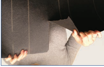
Tar paper provides great "backup" protection under asphalt shingles—but do you really want it as the main waterproofing layer for your tile roof?
