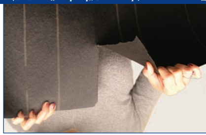
Tar paper provides great "backup" protection under asphalt shingles—but do you really want it as the main waterproofing layer for your tile roof?
