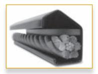
The Impasse™ posts and horizontal rails accept the Stalwart integrated cable system for added perimeter security. This system has successfully tested to the US Department of State K12 rating, stopping a 15,000 pound truck traveling at 50 mph. This system can be used with a variety of vertical materials such as Impasse pales, standard square ornamental pickets, welded wire, etc. to meet site aesthetic requirements. DOS K8 systems also available.
