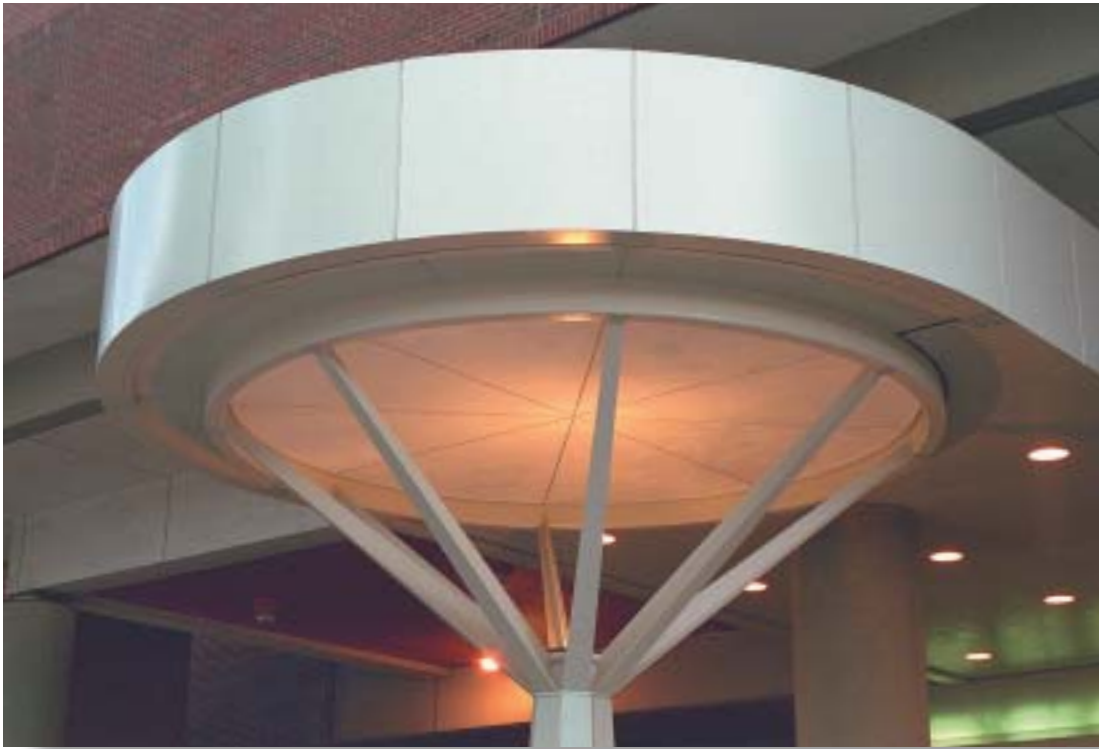
Left: I.B.P. Tech-Clad 1200 curved fascia and soffit in .125" aluminum with Kynar "Ivory" finish.
