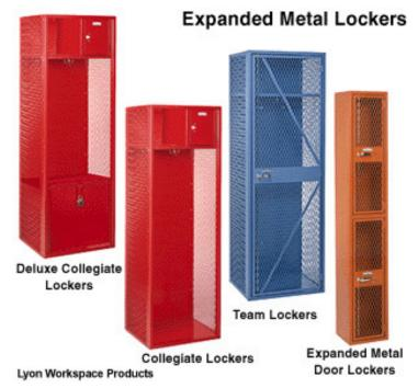
**Material** – Expanded metal shall be 3/4" mesh 13 gauge flattened carbon steel providing approximately 74% open area. Gauges and other steel parts shall be as listed below. Bolts to be zinc plated or subjected to other rust-retardant treatment.
