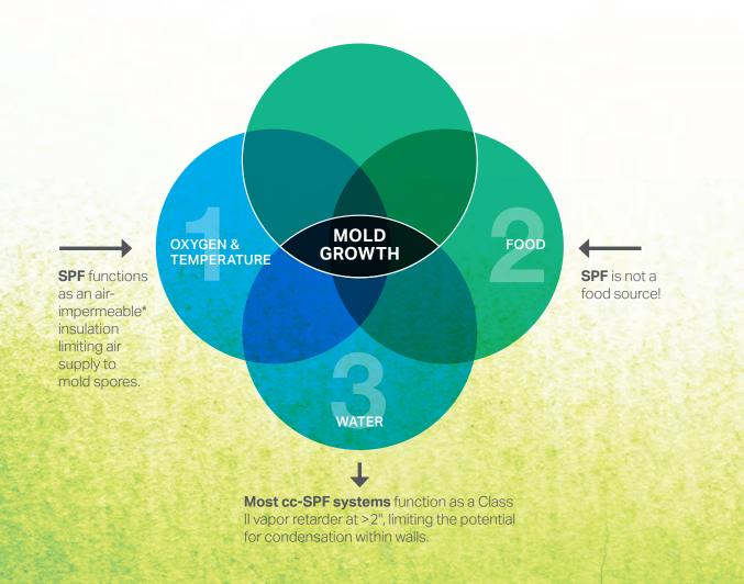
\*AIR-IMPERMEABLE INSULATION as defined by ICC Section R202: An insulation having an air permanence equal to or less than 0.02 L/s-m2 at 75 Pa pressure differential tested according to ASTM E 2178 or E 283.
