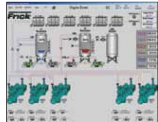
Engine room overview screen
