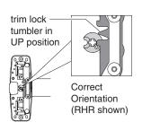
If necessary, remove drive screw and rotate cam until trim lock tumbler is in UP position, then reinstall drive screw
