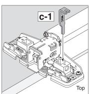
Insert **lift finger screw** and turn clockwise with screwdriver to raise lift finger until the slot aligns with diameter of screw hole.
