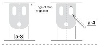
Mark the bottom center point of each slot (a-5) and prepare door frame as shown.
