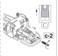
Install retainer clip against lift finger, snapping it into the slot of the **lift finger screw**.
