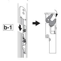
Push bottom latch pin upward. Link will tilt.
