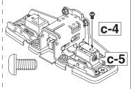
Confirm **lift finger screw** is free to rotate (c-5).
