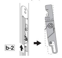
Turn **bottom spool screw** clockwise approximately 20 turns to remove slack. Continue turning until bolt just clears top of strike (b-4).
