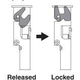
Put top latch in locked position (d-1).
