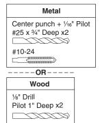
**7b** Install 2 top strike screws using the slot features on the strike.
