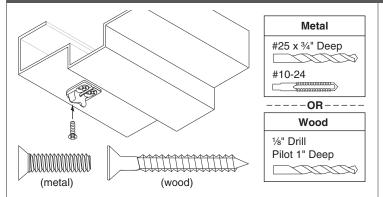
**9b** For fire devices, prepare door edge and cover plate.
