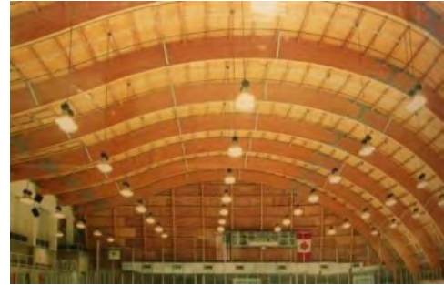
Figure 16: Heavy Timber Construction
