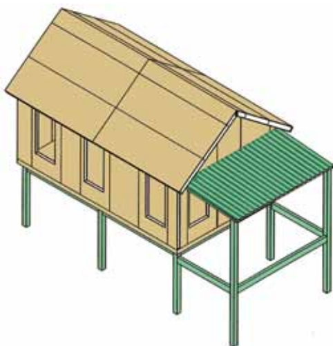
FRONT PORCH WITH METAL ROOF
