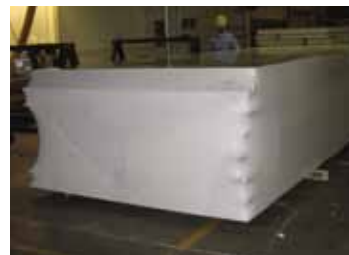
SIPs ARE SHRINK WRAPPED FOR WEATHER PROTECTION
