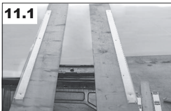
11.1 Attach SIDING-MASTER™ blank rails, 1" x 2" boards, or straight wood stock to 8' x 3/4" boards. Rail legs should face up and sides of rails should be flush along boards. Use 3 – 4 screws to attach blank strip.
