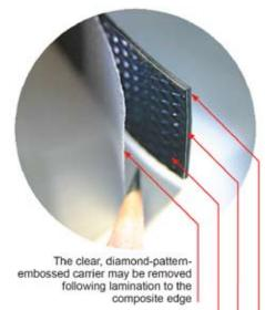
A thinner layer of black polyurethane cushions the edge of the glass composite and accepts the embossed pattern of the carrier through the autoclaving process for an aesthetically pleasing appearance
