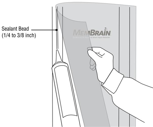
Figure 3: Sealant application.
