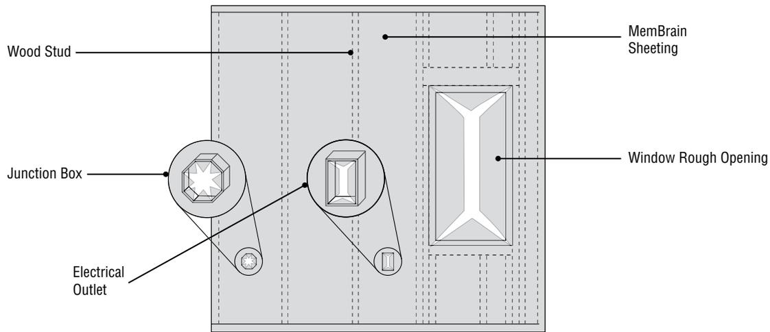
Figure 7: Cut MemBrain sheeting to tightly fit penetrations.
