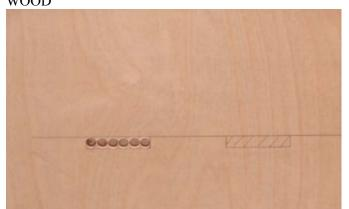
GROOVES ON THE WOOD CAN VERY EASILY BE CUT OUT WITH PLATE JOINTER, IF YOU HAVE ONE, OTHERWISE USE A DRILL WITH 3/8" WOOD BIT. DRILL A FEW HOLES IN THE MARKED AREA 3/4" DEEP.
