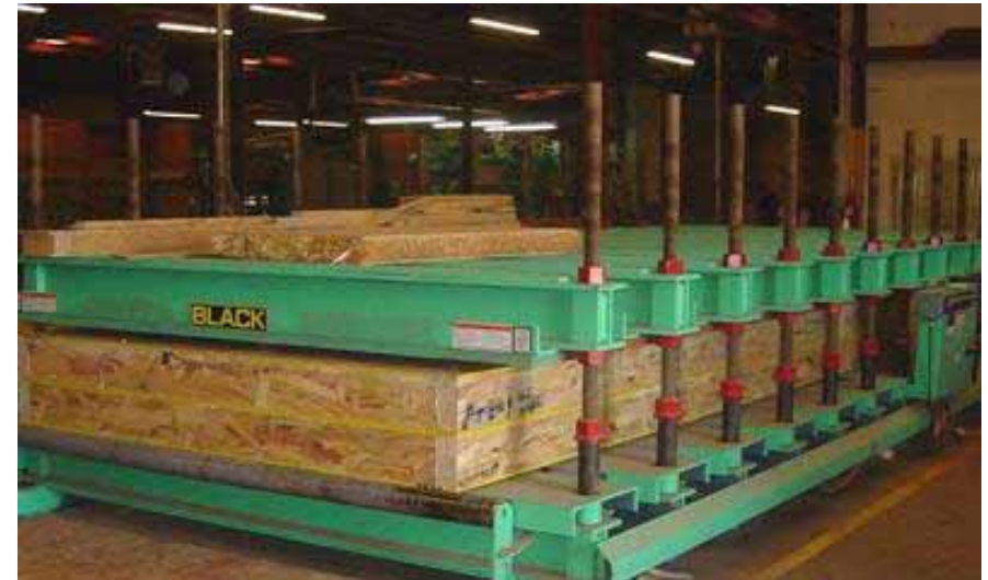
Panel Adhesive Layers Cure in Pod Press
