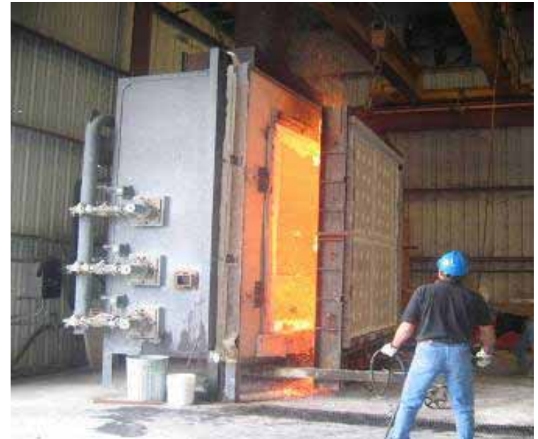
ASTM E-119 Fire Test After 2-1/2 Hr. Exposure
