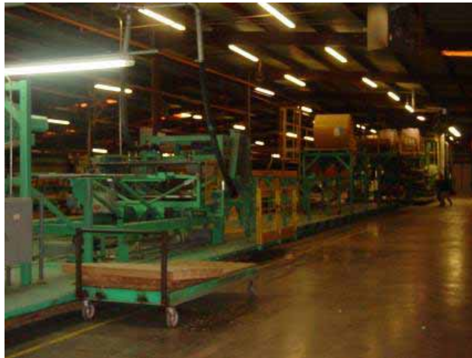
Panel Cutter and Density Checkpoint
