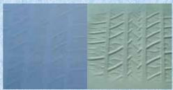
**The Silencer™** (left) even resists indentation from a car's weight, while a competing underlayment (right) may crush permanently, which can cause the floor to sag or buckle.
