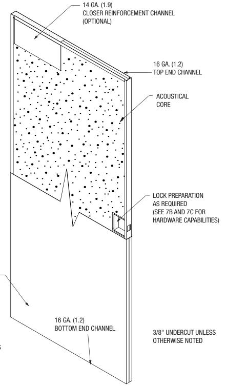
MINIMUM SIZE - 2'0" X 6'8" SINGLE - 4'0" X 6'8" PAIRS MAXIMUM SIZE - 4'0" X 8'0" SINGLE - 8'0" X 8'0" PAIRS
