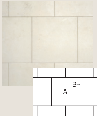
Broken Bond A = 18" x 18" B = 1/8" stripping
