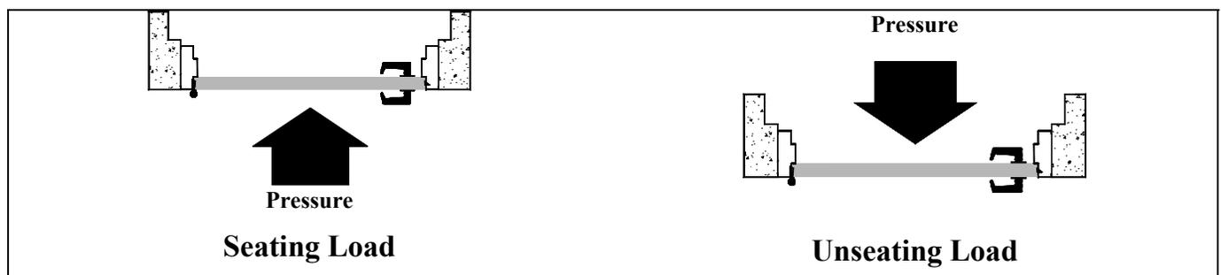
However, if the pressure acts to unseat the door away from the stops, then the hardware must be capable of resisting all loads imposed by the pressure as well as radial and thrust loads. This is an important consideration in the design of both pressure resistant and blast resistant doors, and it has led to the design of special hinges and locking devices.<sup>NB</sup>
