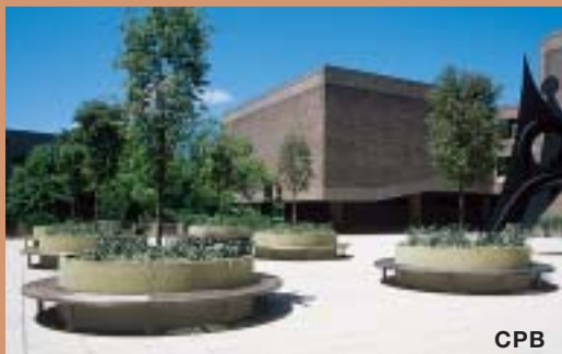
Standard widths: 18"; circular/square planter benches overall d or l 7'-11' Rect. planter benches: overall 48" / min. and 48" w -single, 66" w -double. PLANTER BENCHES
