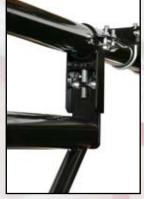
Beam Clamp—Draper's beam clamp provides at least 7 square inches of beam flange contact area and are secured with two all-thread bolts at each attachment point.
