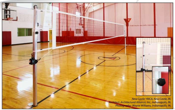
EVS incorporates an internal spring assist mechanism to allow for easy, precise and infinite height adjustment.
