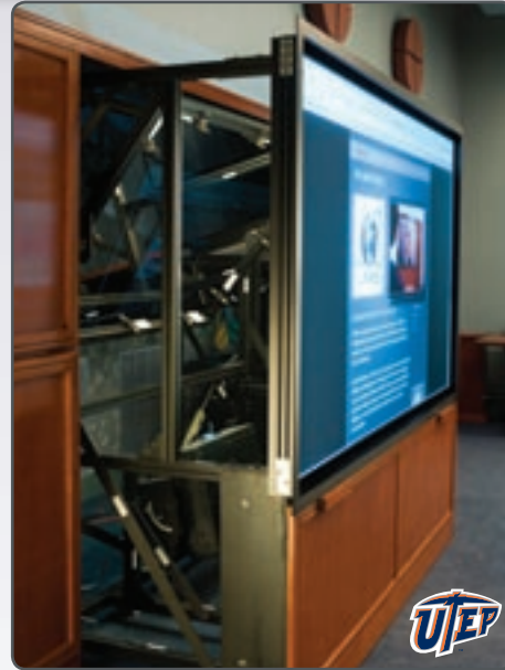
RPX Complete with IRUS screen and Mirror Manager at University of Texas-El Paso. Shown here pulled away from wall for photography. Photography © Graham Hobart, Dallas, TX.
