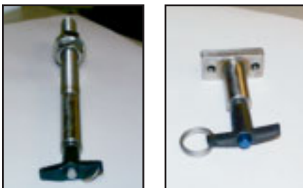
Two types of detent pins. Left photo shows pin typically employed for concrete, stone or similar material. Right photo shows pin typically used for metal window mullion.
