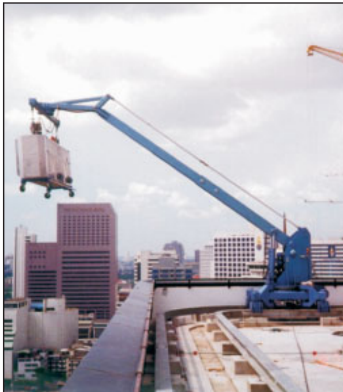
Roof car with traction hoists and wire winders on platform. Platform is 10'-0" (3 m) long.
