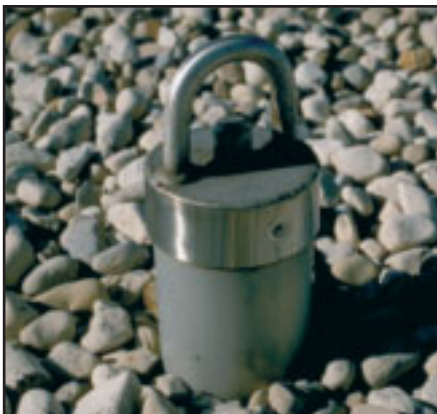
Typical Pro-Bel roof anchor secured to roof structure using any one of a variety of methods e.g. cast-in-place, bolt-through, welding, or chemical adhesive (retrofit). See page G-23 for through-bolt-detail.
