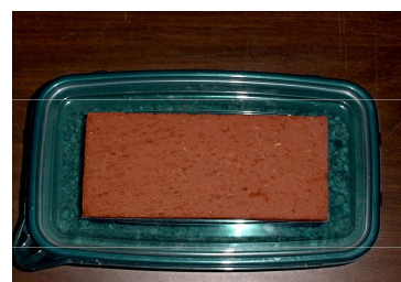
Container Set Up-Efflorescence Test
