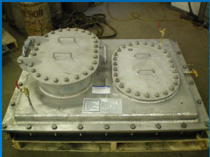
Shock testing manholes
