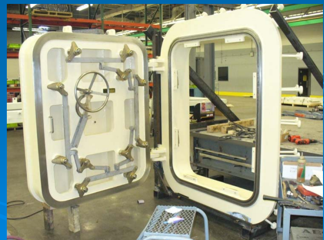
Door designed for 502 psi for dam
