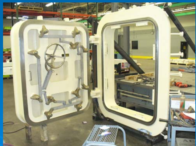
High Pressure watertight door designed for 502 psi & 200 year continuous submersion life for a dam
