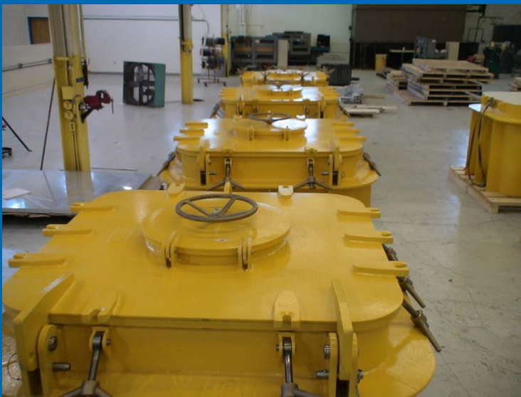
High pressure watertight hatch with counter weight (Model WTH-R)
