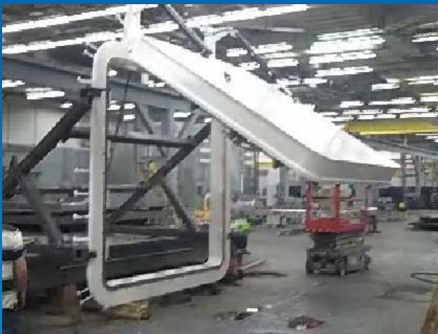
Door designed for 294 psi for mine
