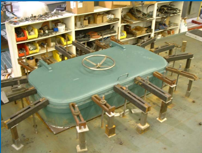
Hydrostatically testing door to 185 psi
