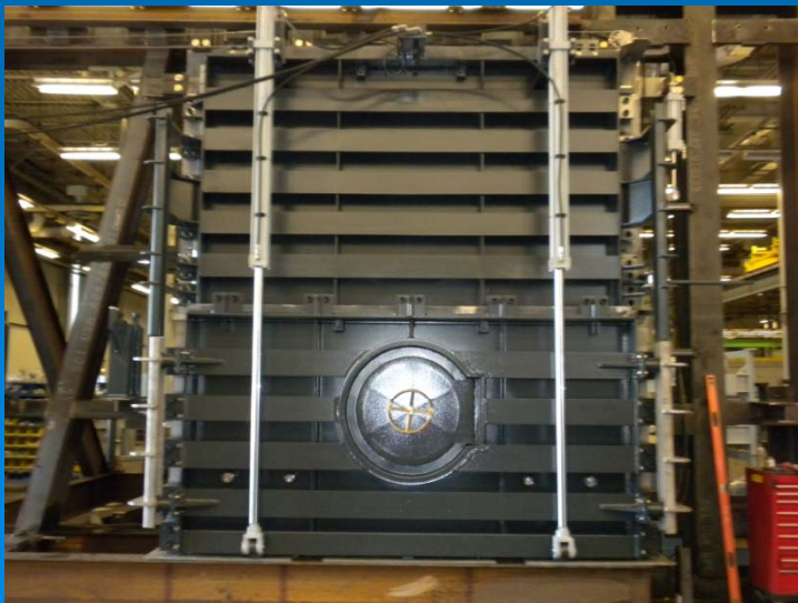
Outage door for nuclear facility during construction
