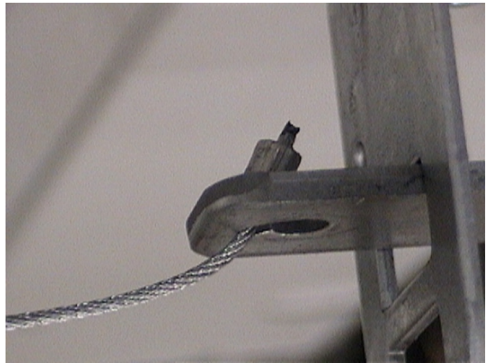
Crimp slug end of cable FIGURE 12
