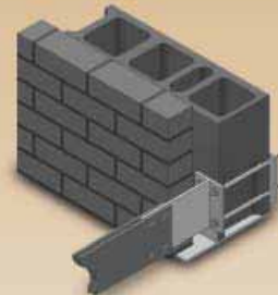
Back Plate Thru-Bolted Through Reinforced Concrete Block
