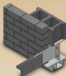
Back Plate Bolted to I-beam
