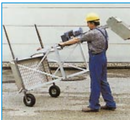
The cradle can be easily moved around using the rollers
