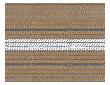
KRAFT PAPER BACKING FOR SPRAY LATH Two strips of Kraft paper 12" wide are factory attached to the lath to conserve the machine applied stucco and to allow visual location of the framing members.
