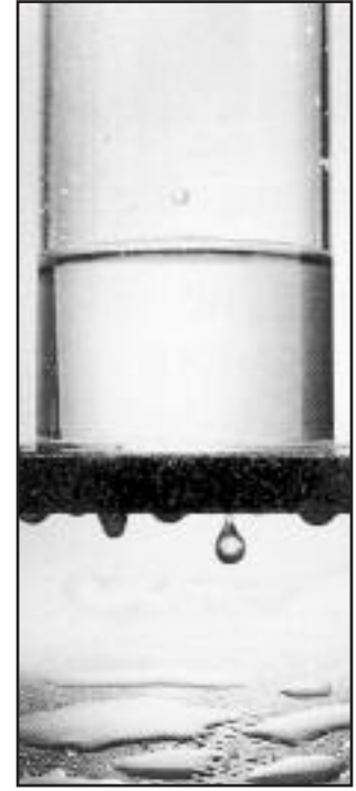
Portland cement board allows moisture to pass through to the wall cavity.
