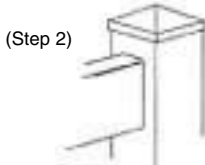
(Step 2) (Top horizontal insertion with dowel and notches)
