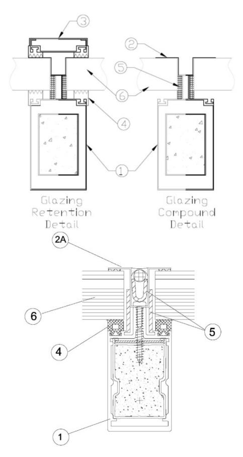
1. Composite Framing Members\* — Nom. 1-15/16 in. wide (50 mm) with a nom. minimum depth of 3-1/8 in. (79 mm) with lengths cut according to glazing size. Perimeter framing members were secured to wall with No. 14 zinc coated or
