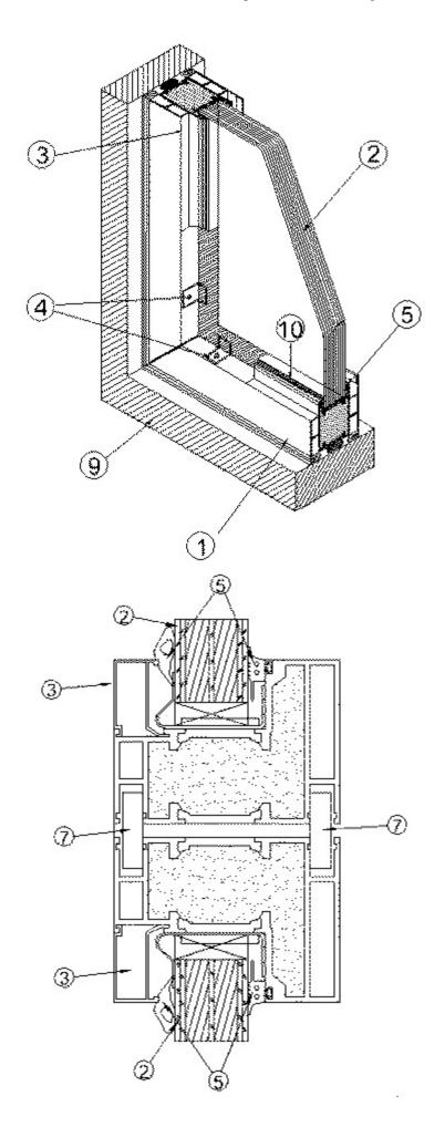
1. **Composite Framing Members\*** — Nom 3.35 in. (85 mm) wide with lengths cut according to glazing opening size. Secured to steel studs with zinc coated TX-30, nominal 2-1/2 in. long self drilling, screws spaced nominally 17 in. OC and 4-1/2 in. from either end.
